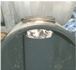
White crystal-like urea deposits clogs the exhaust.
